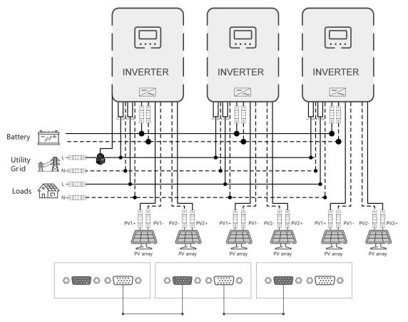
3. Four parallel-connected solar storage inverters:
