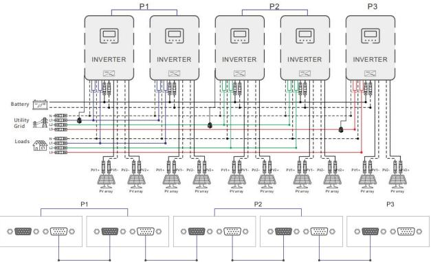
d. Three-phase system (six inverters) 2+2+2 system:
