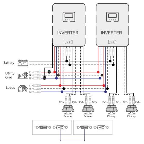
b. Three parallel-connected solar storage inverters:
